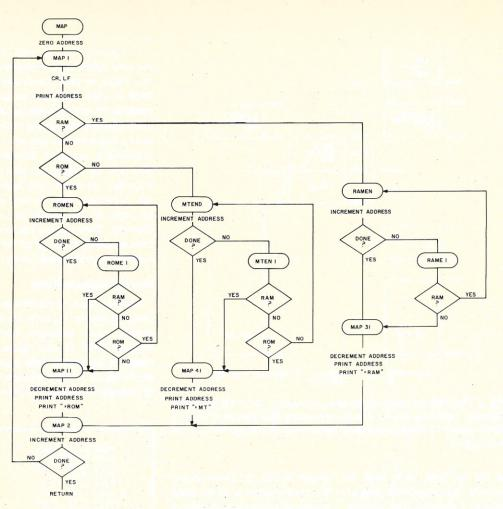
Fig. 4. The flowchart of the Memory Map subroutine, which decides whether a particular memory location contains RAM, ROM or is empty.
